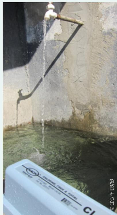
Most commercially available chlorine products are designed to deliver a dose of 2 mg/L in clear water. The recommendation is to double-dose in turbid water (i.e. 4 mg/L). Assuming chlorine demands of 1.5 mg/L in clear water and 3.5 mg/L in turbid water, these doses would be sufficient to maintain at least 0.2-0.5 mg/L of FRC in the treated water.
