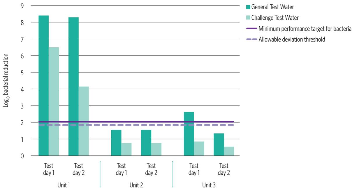
Thus, while the mean log reduction exceeds the performance target of 2  $\log_{10}$ , only one of the three filter units, Unit 1, consistently met or exceeded the performance target.
